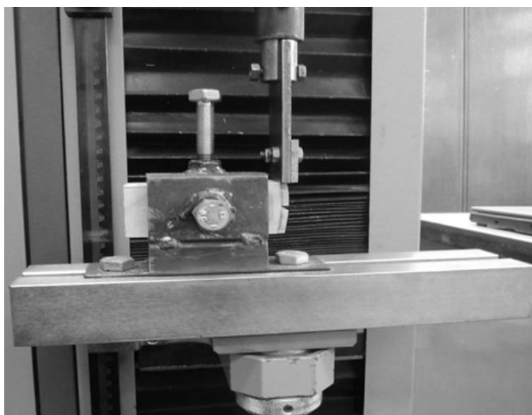
Obr. 6 Testovanie adhézie kôry na dreve. Fig. 6 Wood bark adhesion testing.
