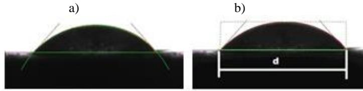
**Fig. 2 Determining the contact angle value by the circle method (a) and by the height-width method (b).**
