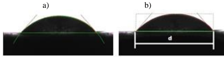
Fig. 2 Determining the contact angle value by the circle method (a) and by the height-width method (b).
