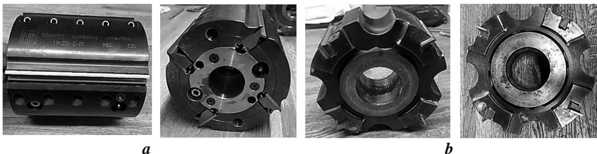
**Fig. 4 Assembled shell-milling cutters that were used on the plano-milling machines during the experimental studies: *a* - on horizontal spindles; *b* - on vertical spindles.**
