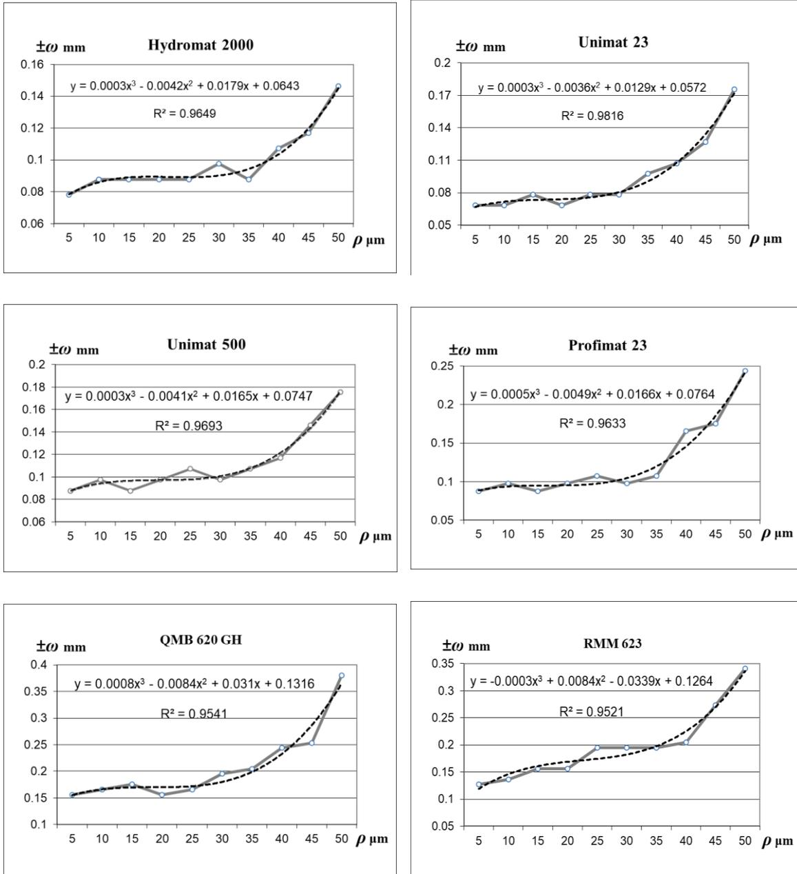
**Fig. 7 Polynomial models of changes in the scattering field of the size of manufactured parts on machine tools.**
