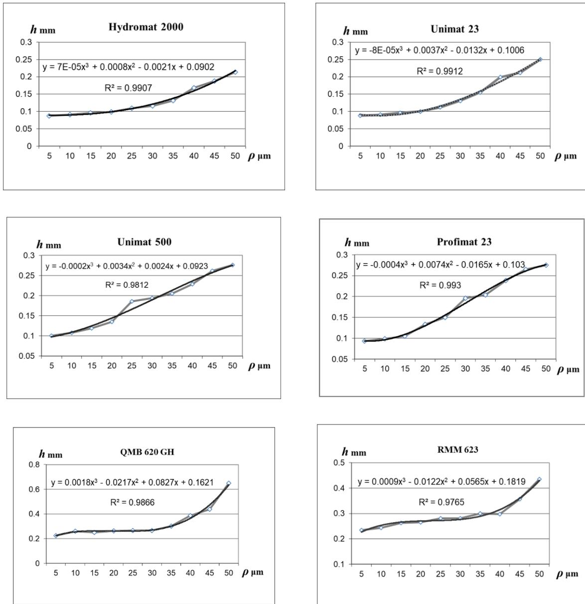
Fig. 6 Polynomial models of changes in the average size of manufactured parts on the machine tools.
