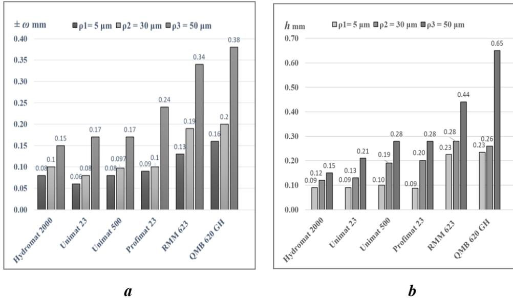
**Fig. 8 Machining accuracy for characteristic phases of the wear resistance period of the milling knives: *a* – by the scattering field; *b* – according to the average value.**
