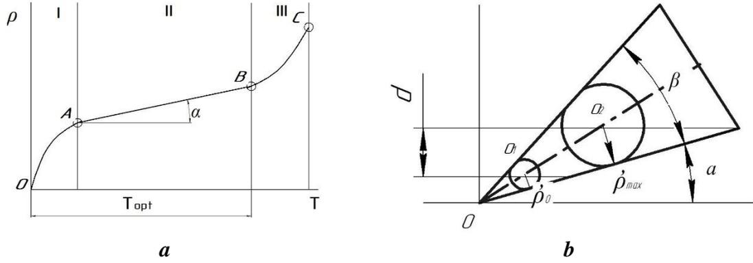
**Fig. 1** Wear and bluntness of wood-cutting tool blades: *a* – the nature of the cutting tool blade wear during operation (Dobryansky and Malafieiev 2020); *b* – changes in the rounding radius of the blades during the cutting tool wear resistance period (Kiryk and Hryhoriev 2013).
