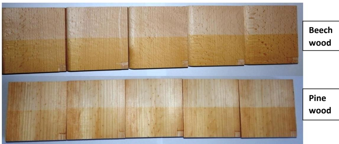
**Fig. 4** Color changes on the pine and beech wood surface during the exposure to UV radiation.
