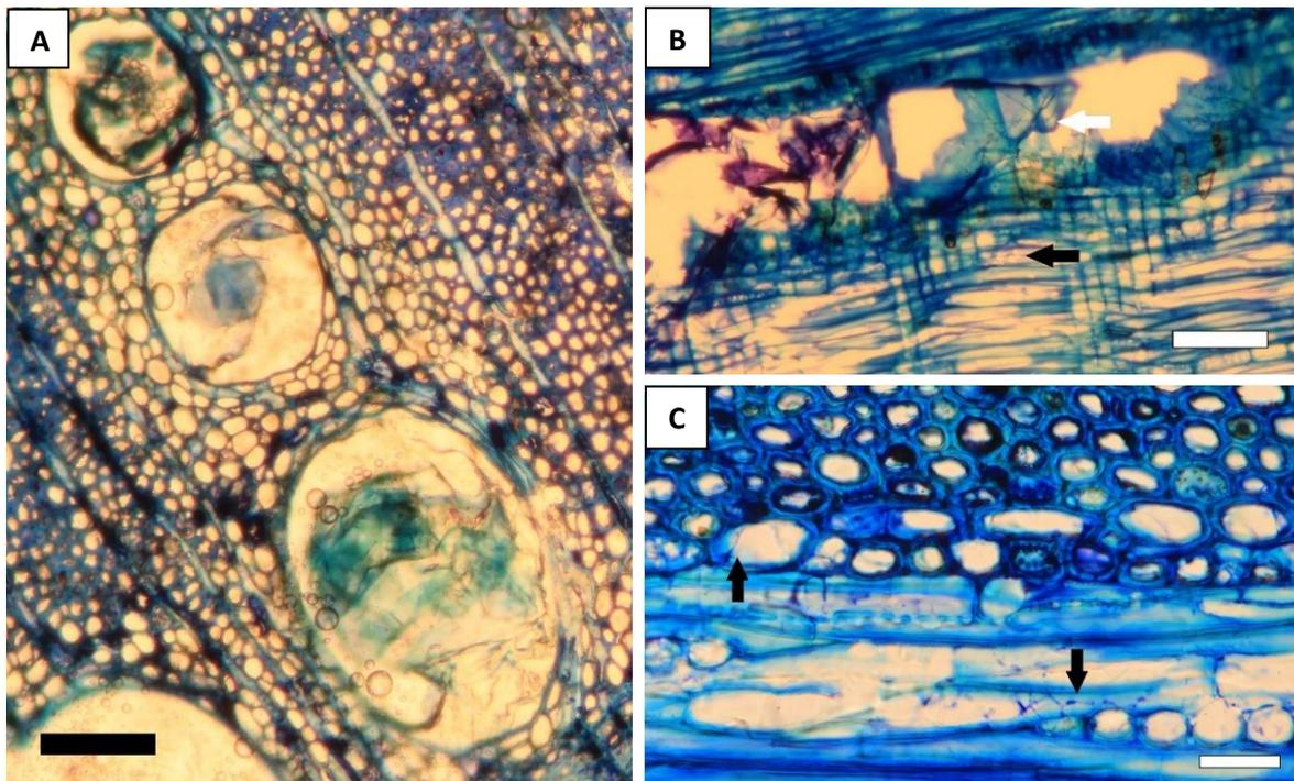
**Fig. 3 Degraded oak heartwood.** The scale equals 50 $\mu\text{m}$  in pictures A and B and 30  $\mu\text{m}$  in picture C, as it is a bigger magnification. Numerous tyloses are visible in picture A. A big tylosis overgrown with hyphae (pointed out with white arrow) is shown in picture A. The black arrow points at bore holes. Picture C shows well-visible hyphae (marked with black arrows). Cell wall disruption is visible as well.
