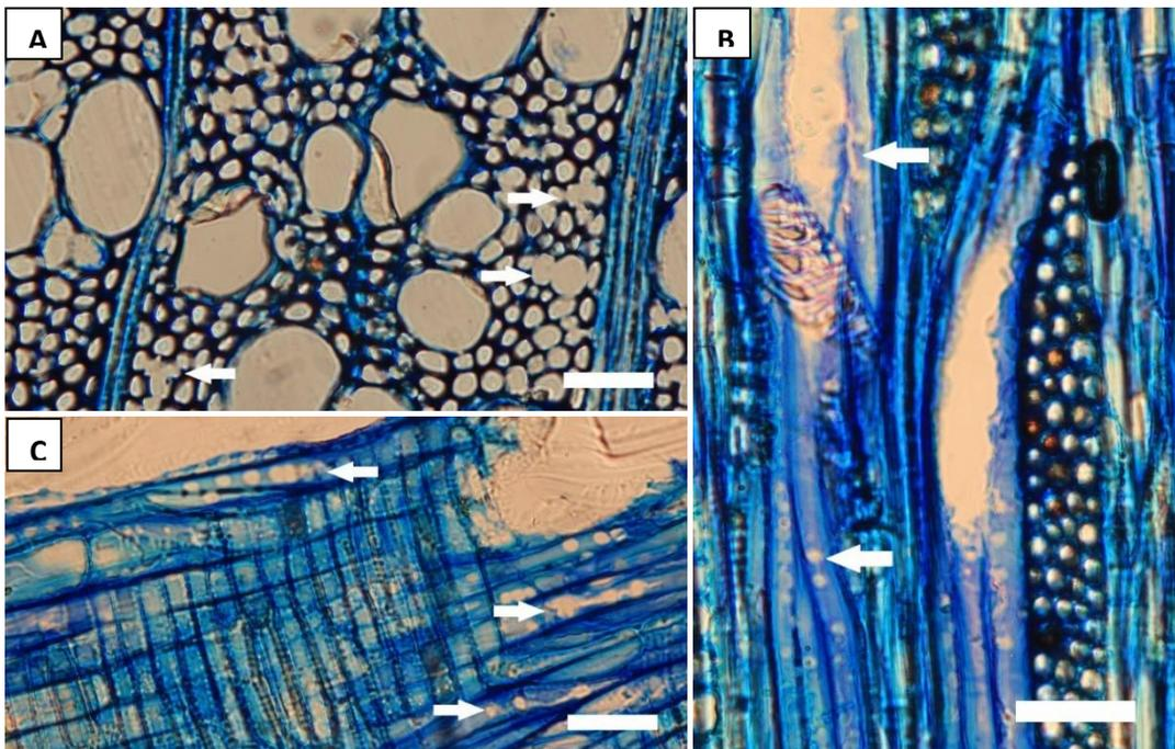
**Fig. 2** Decayed beech wood, scale is marked by white stripes in lower right corner of each image, and it equals to 50  $\mu\text{m}$ . Arrows in picture A show missing or severely disrupted cell walls. Pits in ray parenchyma are more pronounced. Arrows in picture B point at rupture and bore holes in cell walls. Ray parenchyma cells are mostly emptied due to activity of fungus. In picture C, arrows show bore holes turning into big ruptures in cell walls.
