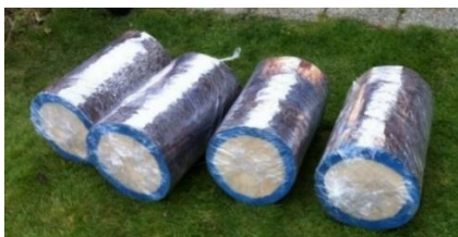
Fig. 1 Sapwood zones in the cross sections of the Norway spruce logs marked by blue colour.
