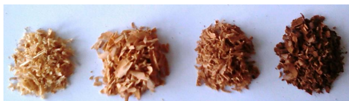
Fig. 2 Samples of the original (0) and steamed oak wood samples (mode I, mode II, mode III).
