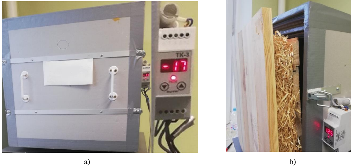
Fig. 3 Laboratory climate chamber (a) with installed fragment of the panel (b).
