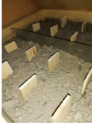
Fig. 4 Container with placed wood samples.
