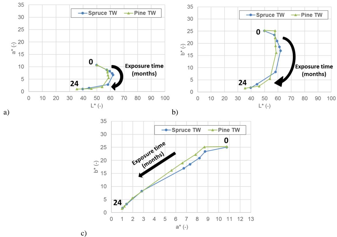
**Fig. 2 Correlations between coordinates of the CIE  $L^*a^*b^*$  colour system for weathered Norway spruce and Scots pine thermally modified woods (TWs).**
