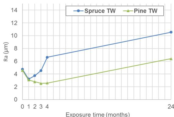
**Fig. 5** Roughness (Ra) of the Norway spruce and Scots pine TWs during natural weathering.
