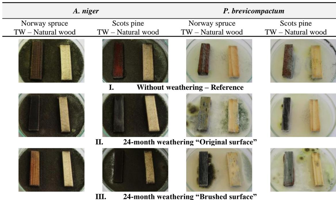
**Fig. 6.** The mould growth activity (MGA) of two microscopic fungi evaluated after 4 days on the top surfaces of the Norway spruce and Scots pine TWs and natural wood.
