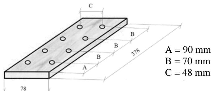
**Fig. 1 Measurement points on samples for the analysis of the colour, gloss, and roughness.**
