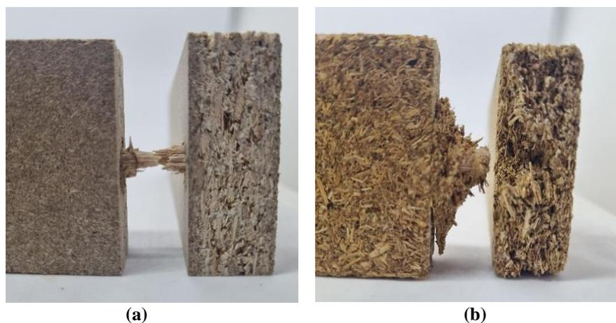
**Fig. 4 Failure modes in some of the studied cases – wooden dowel at:
