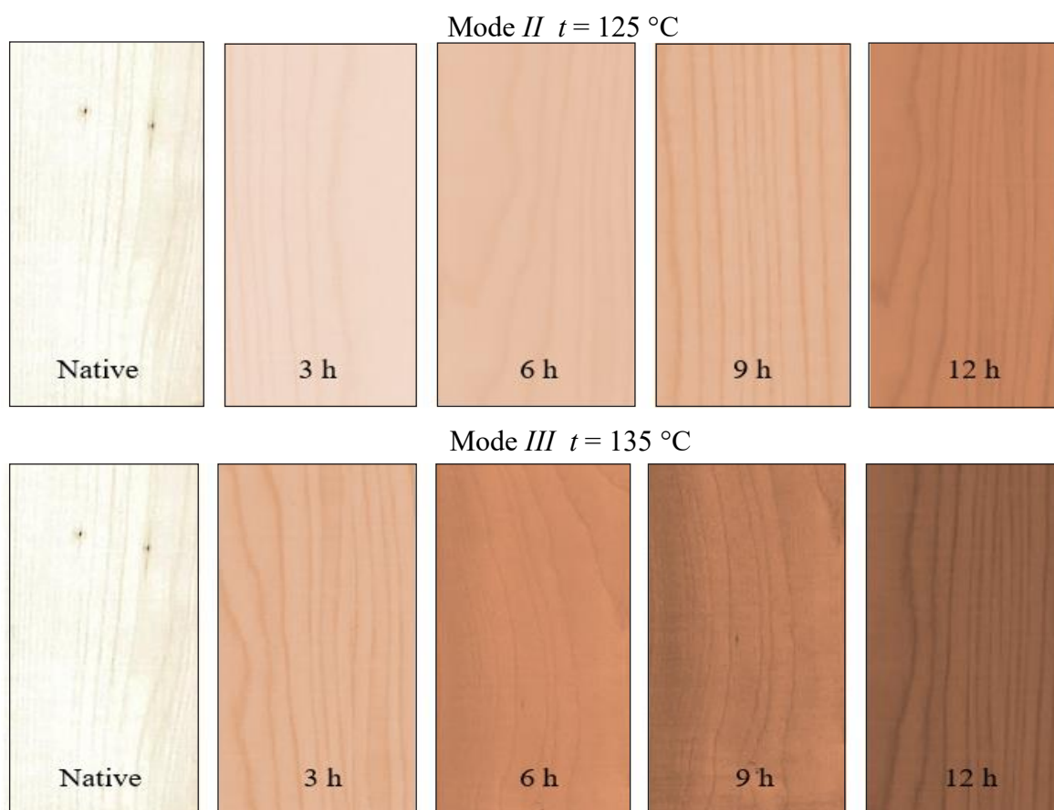
Fig. 2 Changes in the colour of maple wood during the process of thermal treatment
