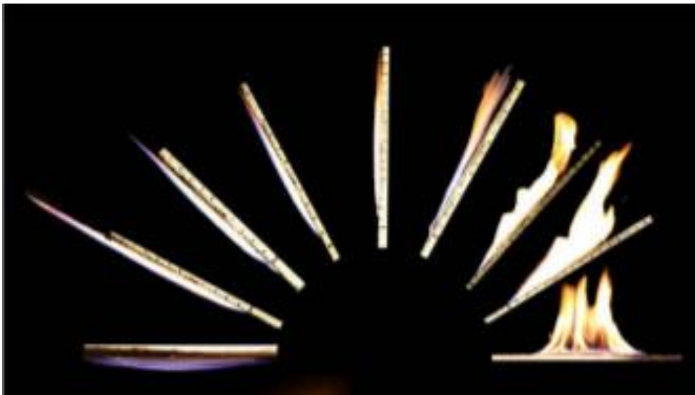
Fig. 1. Flame propagation at different angles of inclination (GOLLNER et al. 2017).
