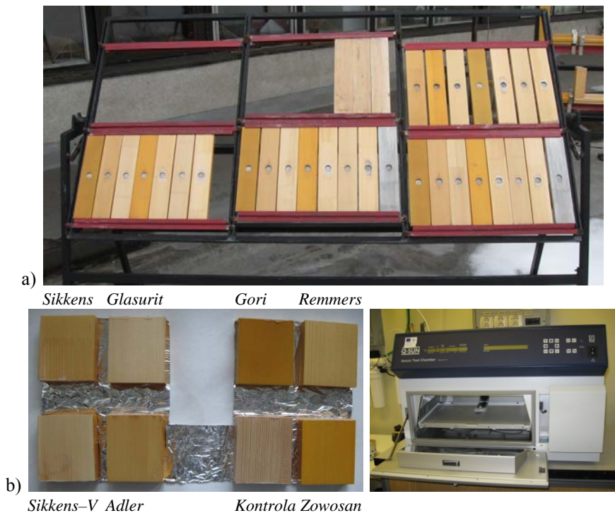
Obr. 2 Starnutie telies v exteriéri po 9 mesiacoch (a) a v Xenoteste po 3 týždňoch (b). Fig. 2 Ageing of samples in exterior after 9 months (a) and in Xenotest after 3 weeks (b).
