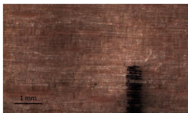
Fig. 5 The intrusion on Hard wax surface finish with three layers at a drop height of 400 mm.
