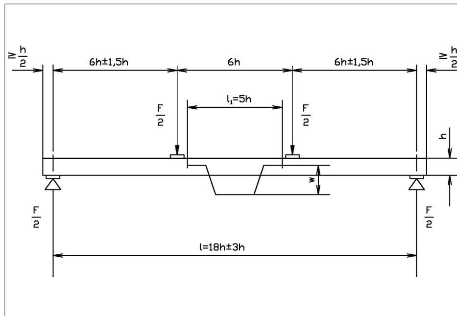
Fig. 3 Four-point bending test arrangement (ČSN EN 408).
