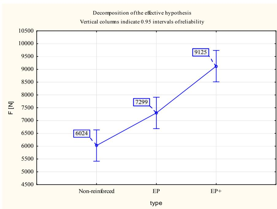
**Fig. 4 Dependence of the loading force according to the beam types.**
