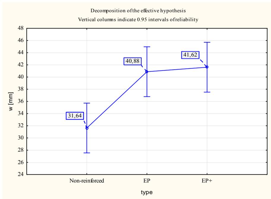
**Fig. 5 Flexure dependence according to the beam types.**
