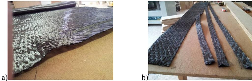
**Fig. 1 SikaWrap 300 carbon fabric used for reinforcing a) delivered condition b) created individual strips according to the beam dimension.**
