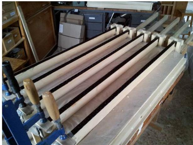
**Fig. 2 Attaching the pre-strained carbon fabrics to the wood beams.**
