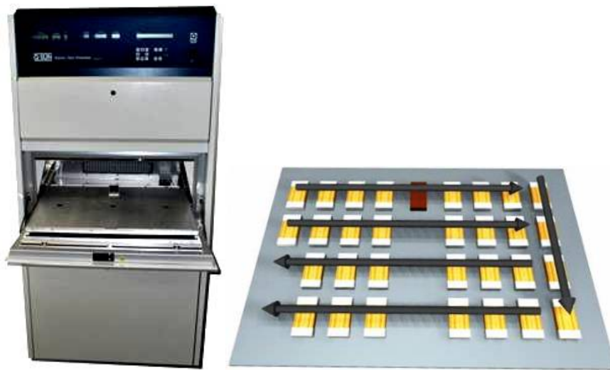
Fig. 1 Equipment Q-SUN Xe-3-HS and specimens' rotation during accelerated ageing
