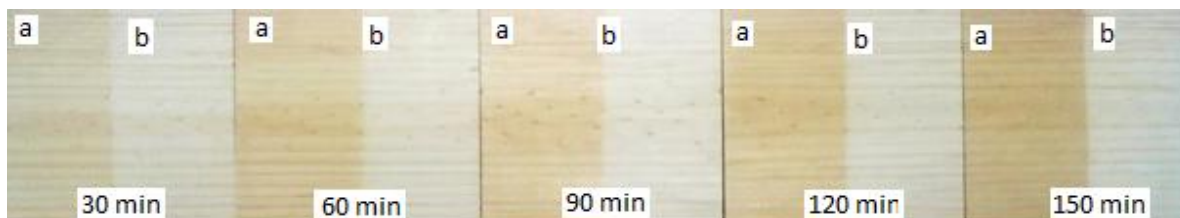
Fig. 1 Colour changes on the spruce wood surface during the exposure to UV irradiation (a - exposed surface, b - unexposed surface).
