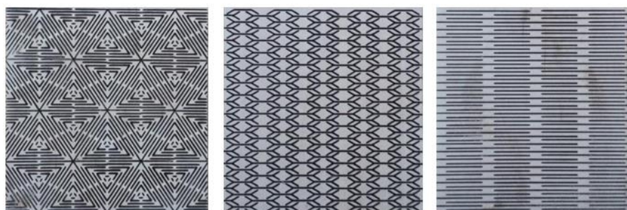
Fig. 2 Perforations used to increase material formability; they also fulfill an aesthetic function (OBRARY, s. a.).
