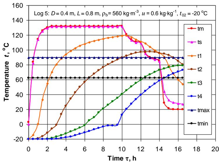
**Fig. 6** Change in  $t_m$ ,  $t_s$ , and  $t$  in 4 representative points of the Log 5 with  $t_{o2} = -20$  °C during its steaming in an autoclave and its subsequent conditioning at  $t_{air} = 20$  °C.
