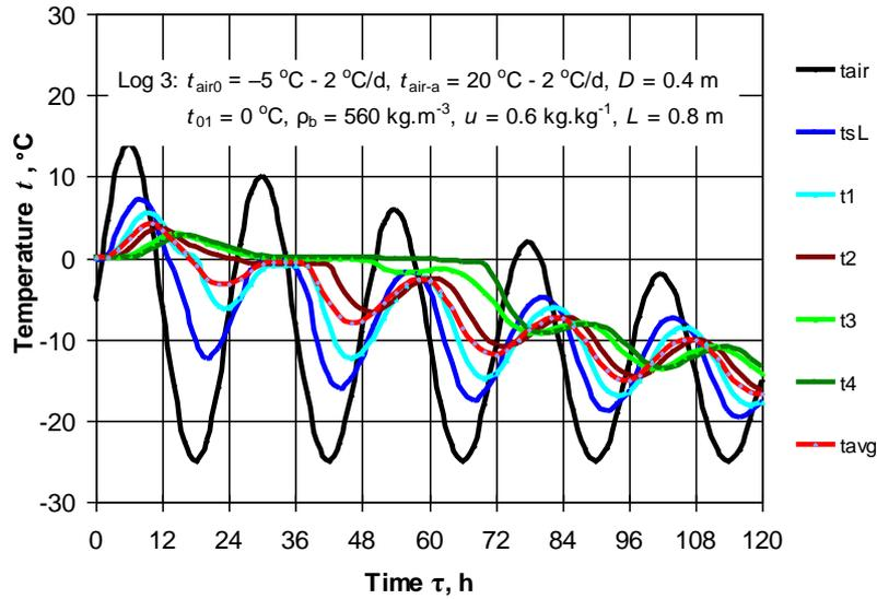
**Fig. 4 Change in  $t_{air}$ ,  $t_s$ ,  $t_{avg}$ , and  $t$  of 4 representative points of the Log 3 during its 120 h periodical freezing and defrosting at decreasing values of  $t_{air0}$  and  $t_{air-a}$ .**
