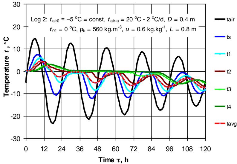
**Fig. 3** Change in  $t_{air}$ ,  $t_s$ ,  $t_{avg}$ , and  $t$  of 4 representative points of the Log 2 during its 120 h periodical freezing and defrosting at constant value of  $t_{air0}$  and decreasing value of  $t_{air-a}$ .
