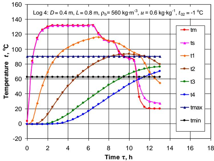
**Fig. 5** Change in  $t_m$ ,  $t_s$ , and  $t$  in 4 representative points of the Log 4 with  $t_{o2} = -1$  °C during its steaming in an autoclave and its subsequent conditioning at  $t_{air} = 20$  °C.
