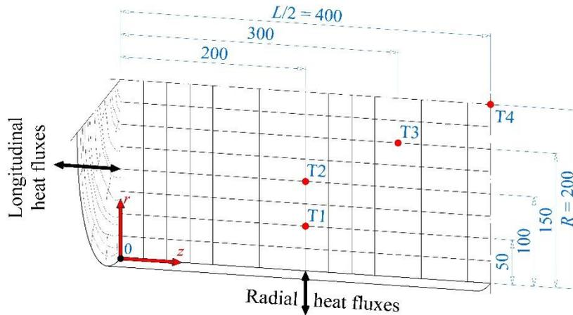
**Fig. 1 Positioning of the coordinate axes and the knots of the calculation mesh with representative points T1, T2, T3, and T4 on  $\frac{1}{4}$  of the longitudinal section of log subjected to freezing, defrosting, and autoclave steaming.**
