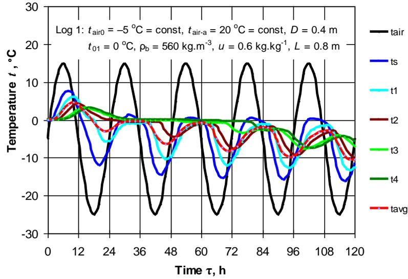
**Fig. 2** Change in  $t_{air}$ ,  $t_s$ ,  $t_{avg}$ , and  $t$  of 4 representative points of the Log 1 during its 120 h periodical freezing and defrosting at constant values of  $t_{air0}$  and  $t_{air-a}$ .
