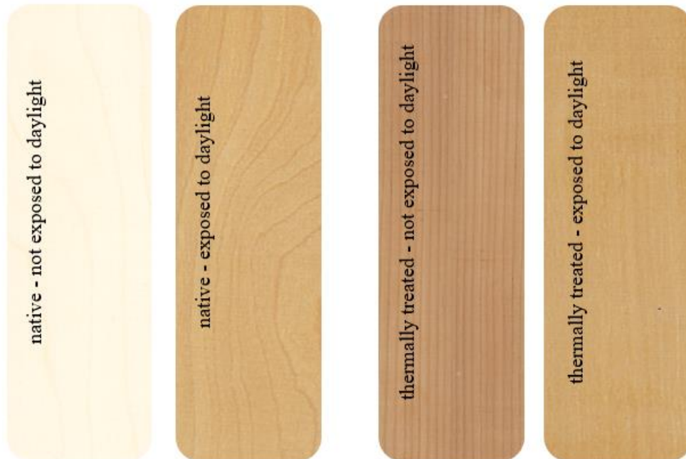
Fig. 2 View of maple wood: native before and after exposure; thermally treated before and after exposure.
