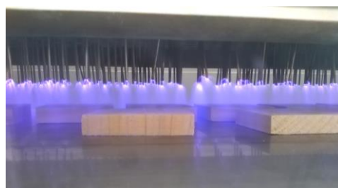
Obr. 2 Predúprava telies smreka plazmou v prístroji ADRE plasma. Fig. 2 Pretreatment of the spruce samples in the ADRE plasma device.
