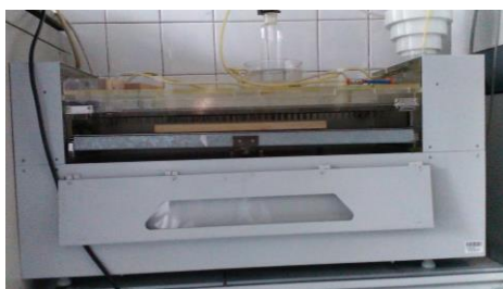
Obr. 2 Predúprava telies smreka plazmou v prístroji ADRE plasma. Fig. 2 Pretreatment of the spruce samples in the ADRE plasma device.
