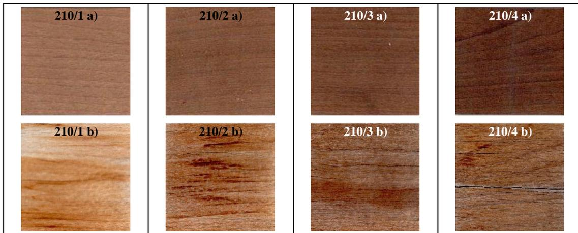
**Fig. 6** The colors of the beech wood specimens thermally modified in air at 190 °C and 210 °C during 1–4 hours (a), and the color changes together with the longitudinal cracks created at the 6-weeks weathering in Xenotest (b).
