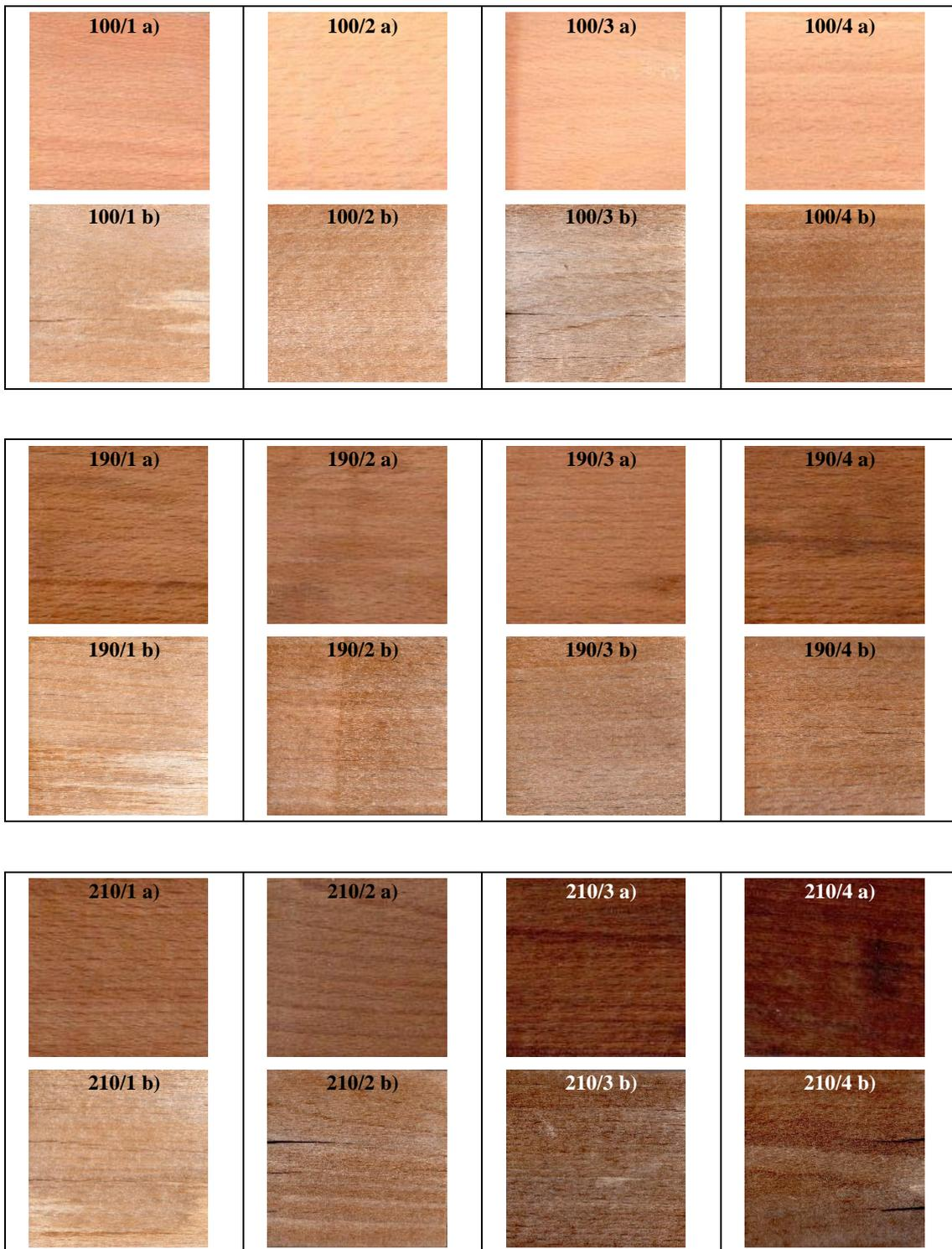
**Fig. 7** The colors of the beech wood specimens thermally treated in paraffin at 100 °C, 190 °C and 210 °C during 1 – 4 hours (a), and the color changes (for the hardest modification modes “210 °C/2–4h” as well as the longitudinal cracks) created at the 6-weeks weathering in Xenotest (b).
