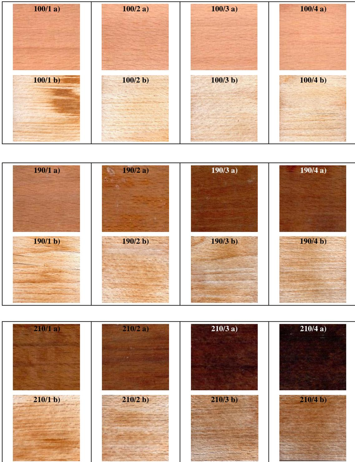
**Fig. 8** The colors of the beech wood specimens thermally treated in PEG 6000 at 100 °C, 190 °C and 210 °C during 1 – 4 hours (a), and the color changes created at the 6-weeks weathering in Xenotest (b).
