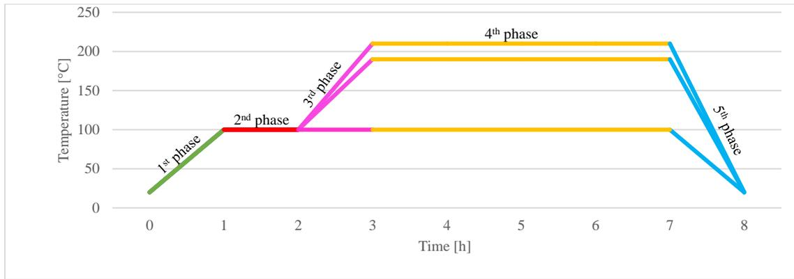
**Fig. 1 Phases of the thermal treatment of beech wood in air, paraffin or PEG 6000.**
