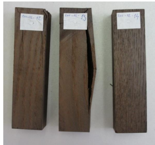
Fig. 5 The failure of samples treated by the temperature of 200 °C for 12 hours.
