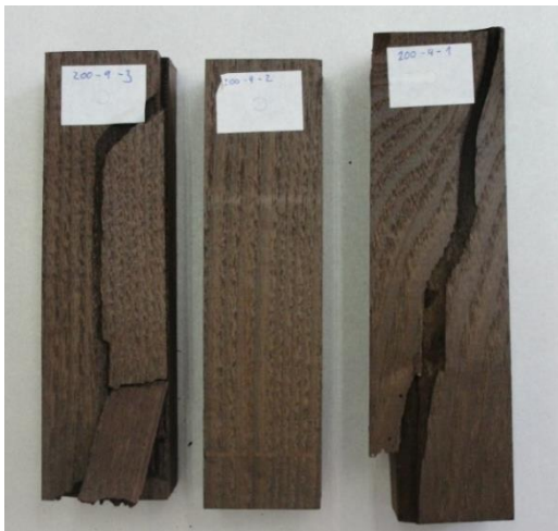
Fig. 4 The failure of samples treated by the temperature of 200 °C for 9 hours.
