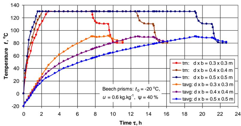
**Fig. 4** Change in  $t_m$  and  $t_{avg}$  during the steaming of beech prisms with  $t_0 = -20\text{ }^\circ\text{C}$  in an autoclave at  $\gamma = 40\%$ , depending on their cross-section dimensions.
