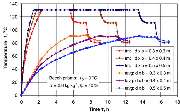
**Fig. 3** Change in  $t_m$  and  $t_{avg}$  during the steaming of beech prisms with  $t_0 = 0\text{ }^\circ\text{C}$  in an autoclave at  $\gamma = 40\%$ , depending on their cross-section dimensions.
