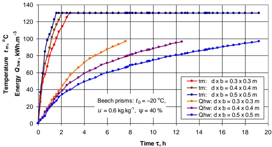
**Fig. 6** Change in  $t_m$  and  $Q_{hw}$  during the steaming of beech prisms with  $t_0 = -20\text{ °C}$  in an autoclave at  $\gamma = 40\%$ , depending on their cross-section dimensions.
