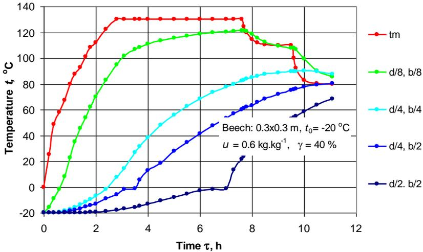
**Fig. 2** Change in  $t_m$  and  $t$  in 4 characteristic points of beech prisms with cross-section dimensions  $d \times b = 0.3 \times 0.3$  m and  $t_0 = -20$  °C during their TTP in an autoclave at a loading of 40%.
