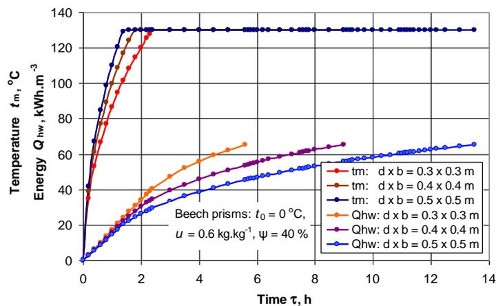
**Fig. 5** Change in  $t_m$  and  $Q_{hw}$  during the steaming of beech prisms with  $t_0 = 0\text{ }^\circ\text{C}$  in an autoclave at  $\gamma = 40\%$ , depending on their cross-section dimensions.
