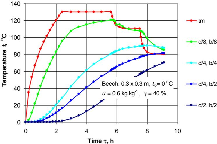
**Fig. 1** Change in  $t_m$  and  $t$  in 4 characteristic points of beech prisms with cross-section dimensions  $d \times b = 0.3 \times 0.3$  m and  $t_0 = 0$  °C during their TTP in an autoclave at a loading of 40%.
