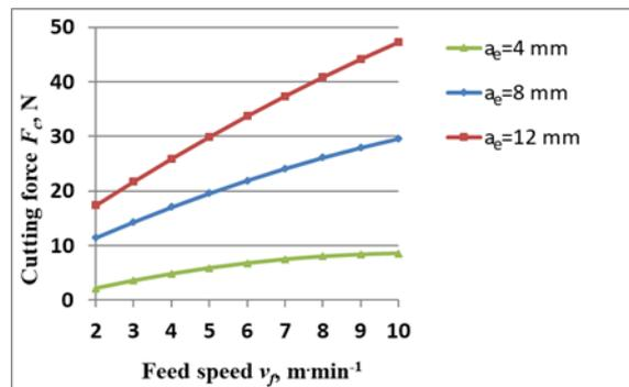
Fig. 4.5 Influence of feed speed at different uncut chip thicknesses when milling plywood.
