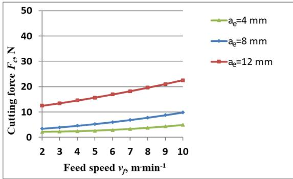
Fig. 4.3 Influence of feed speed at different uncut chip thicknesses when milling oak.
