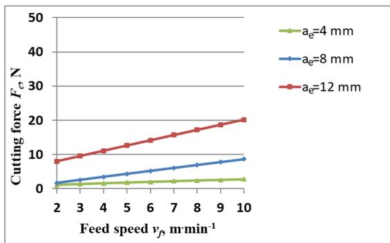
**Fig. 4.1 Influence of feed speed at different uncut chip thicknesses when milling meranti.**
