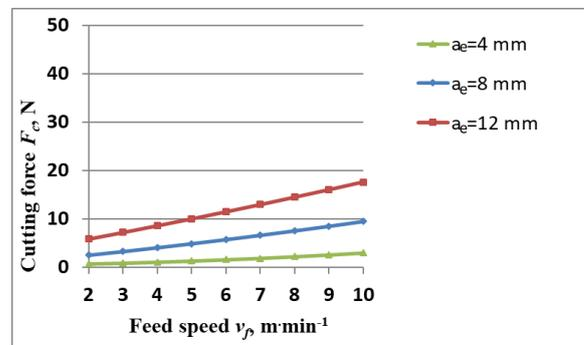
**Fig. 4.2 Influence of feed speed at different uncut chip thicknesses when milling koto.**
