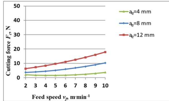
Fig. 4.4 Influence of feed speed at different uncut chip thicknesses when milling MDF.
