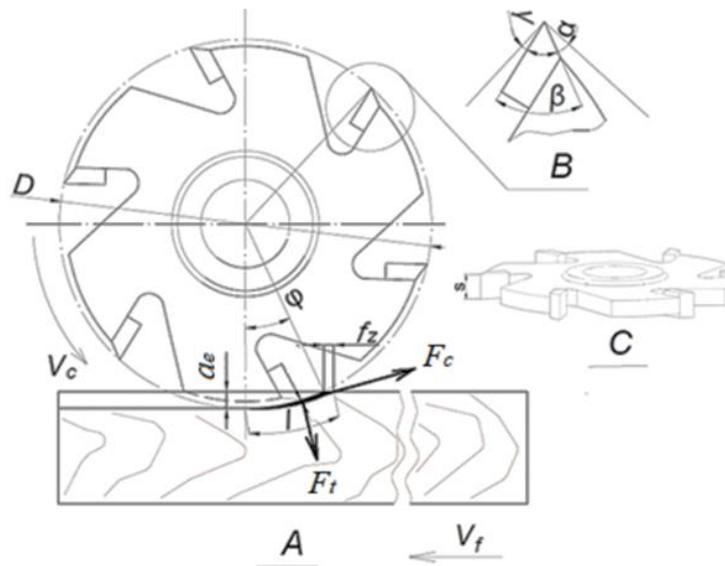
Fig. 1 Basic cutting against the feed parameters.
