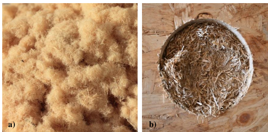
Fig. 2 Wood fibres STEICO zell (a) and disintegrated straw stalks TEPORE (b).
