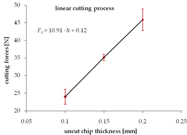
Fig. 3 Cutting force versus uncut chip thickness when orthogonal linear cutting pine wood.
