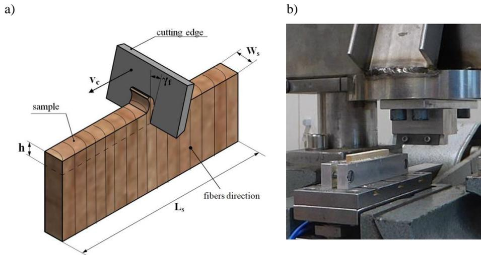
**Fig. 1 Orthogonal linear cutting process: a) schema of cutting process, b) microtome instrument while cutting.**
