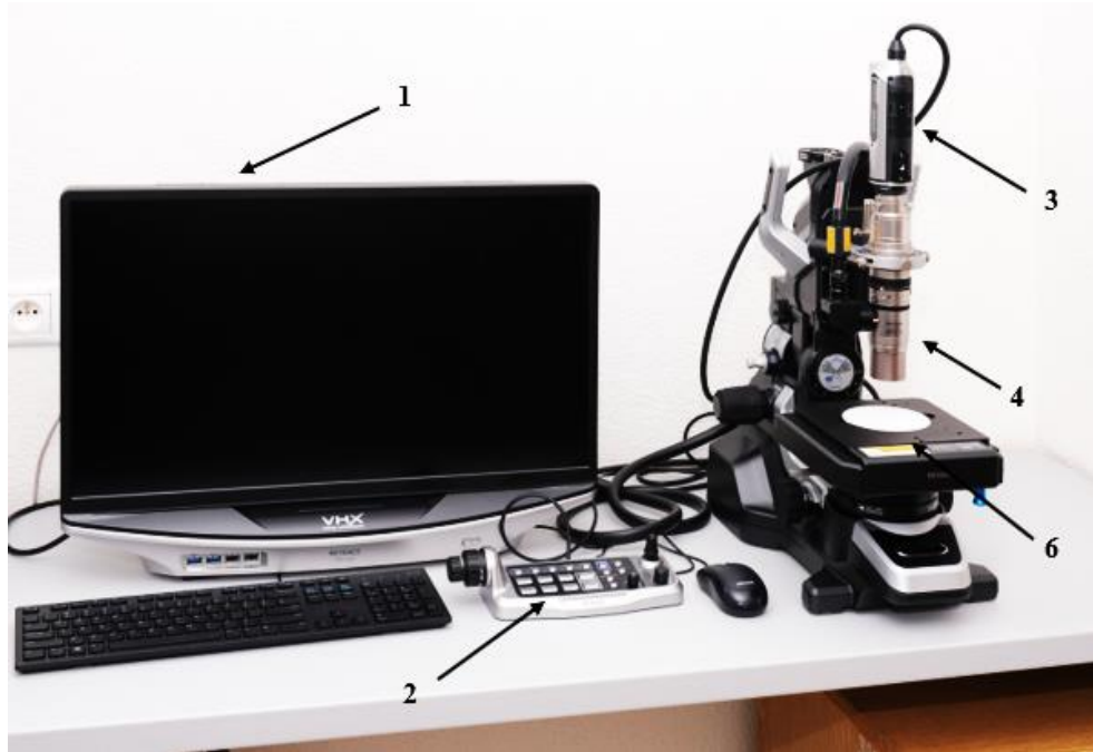
Fig. 2 Construction of the Keyence VHX-7000 digital microscope.
