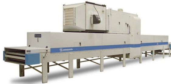
Fig. 1 General view of equipment for unilateral convective heating of furniture elements before their subsequent lacquering.
