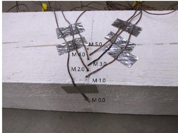
**Fig. 1** Emplacement of the thermocouples M 0.0 – M 5.0.
