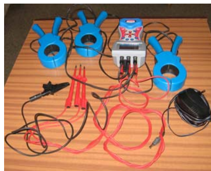
Obr. 5 Metrel Power Q Plus MI 2392 Fig. 5 Metrel Power Q Plus MI 2392
