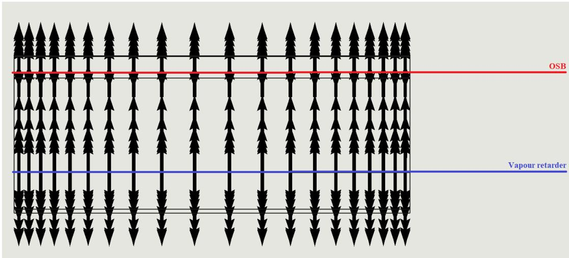
Fig. 6 Diffusion flux direction S2C in November – from ZELL to OSB (WUFI2DMotion).
