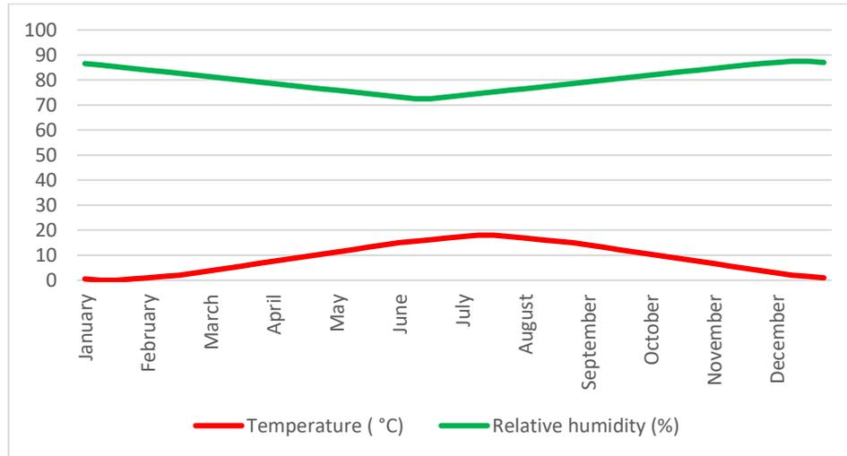
**Fig. 4 Boundary conditions on the exterior side of the structure during year.**
