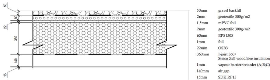
**Fig. 1 Structure composition of wood-based compact flat roof with gravel backfill, versions S1A-C (version A – vapour barrier  $S_a=300m$ ; version B – vapour retarder  $S_a=0.3-5m$ ; version C – vapour retarder  $S_a=0.5-30m$ )(author).**
