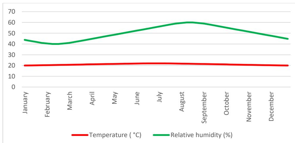
**Fig. 3 Boundary conditions on the interior side of the structure during year.**
