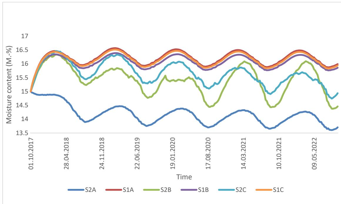
**Fig. 9 The moisture content of the OSB – oriented strand board.**
