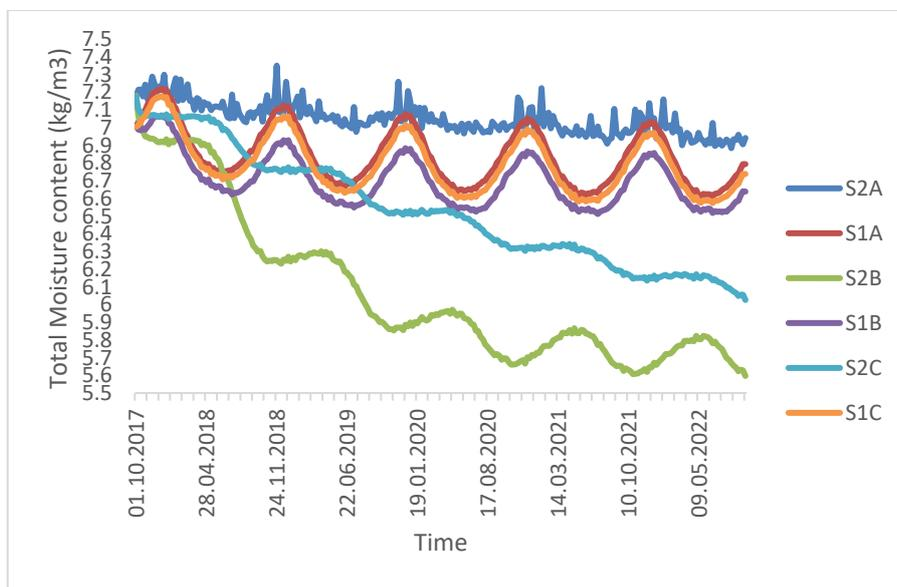
**Fig. 5 Total moisture content in fragments of compact flat roof [kg/m<sup>3</sup>].**
