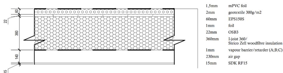
**Fig. 2 Structure composition of wood-based compact flat roof without gravel backfill, versions S2A-C (version A – vapour barrier  $S_a=300m$ ; version B – vapour retarder  $S_a=0.3-5m$ ; version C – vapour retarder  $S_a=0.5-30m$ )(author).**
