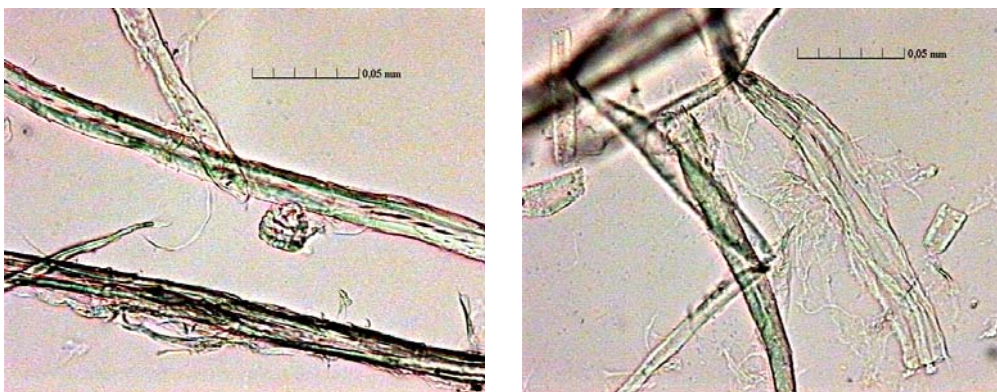
Obr. 1 Zmeny vlákien – fibrilácia v procese mletia [6] Fig. 1 The changes of fibers – the fibrillation in the beating process
