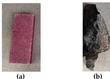
**Fig. 13 Sample of fire-proof board before (a) and after (b) testing.**
