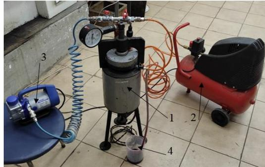
**Fig. 6** The general arrangement of the test bench: 1: autoclave; 2: compressor; 3: vacuum pump; 4: fire retardant reservoir.
