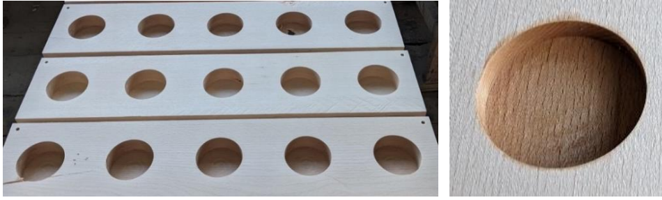
Fig. 1 On the left – sample plank with cut openings. On the right – opening after application of the penetrating coating.
