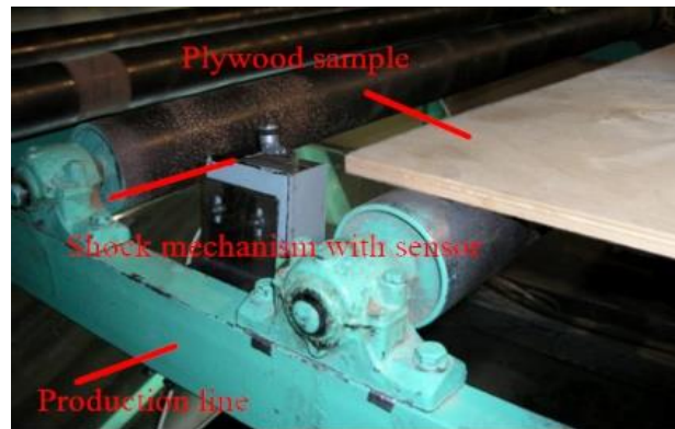
Fig. 4 Approbation device for defect control.
