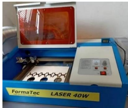
Fig. 1. CO<sub>2</sub> laser machine for engraving and cutting.
