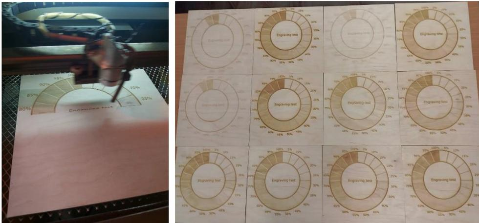
**Fig. 3. Results of an engraving test and changes in the colour of birch plywood.**
