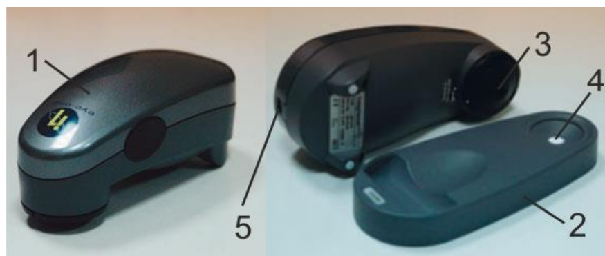
Fig. 3 Spectrophotometer GretagMacbeth “Eye-One Pro”: 1 – measuring device; 2 – platform; 3 – light source; 4 – white plate; 5 – Mini Display port for PC connection.
