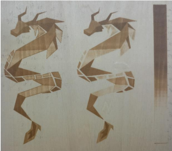
Fig. 8 Engraved images: a – with the key line; b – without the key line.
