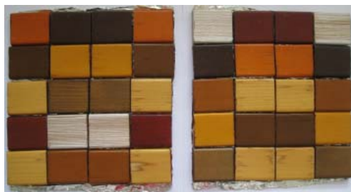
Obr. 1 Telesá smreka s nátermi “Sokrates” starnuté prirodzene (a) a v Xenoteste (b). Fig. 1 Spruce samples with “Sokrates” paints aged naturally (a) and in Xenotest (b).
