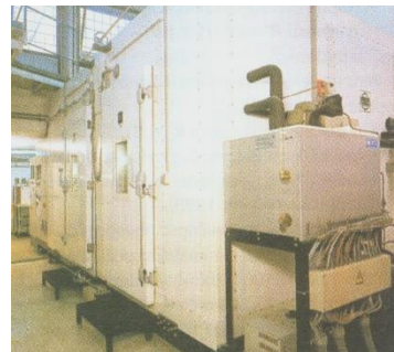
Obr. 2 Schéma laboratórneho zariadenia veľkej klíma komory. Fig. 2 Scheme of laboratory equipment large climate chamber.
