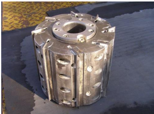
Fig. 2 The milling head with hydraulic clamping without back fixation of planing blades.
