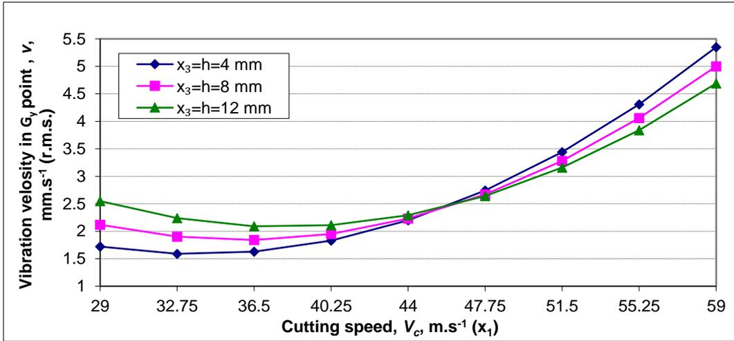
Fig. 7 Changes in the vibration velocity  $v$  at measurement point  $G_y$  in relation to the cutting speed  $V_c$  at different out-cut layers  $h$ .
