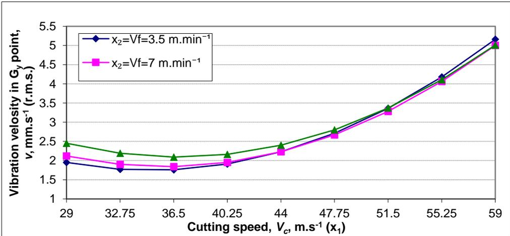
Fig. 6 Assessment of vibration velocity  $v$  at measurement point  $G_y$  in relation to the cutting speed  $V_c$  at different feed speed  $V_f$ .
