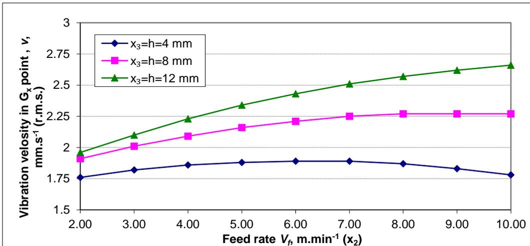
Fig. 8 Changes in vibration velocity  $v$  at measurement point  $G_x$  in relation to the feed speed  $V_f$  at different thicknesses of the out-cut layer  $h$ .
