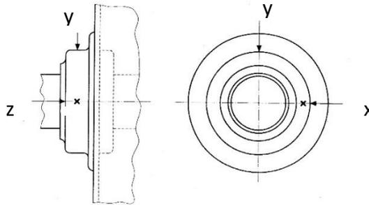
**Fig. 3 Measurement points on one bearing housing.**
