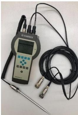
**Fig. 4 General view of the vibration meter, model *Vibrotest 60*, equipped with acceleration sensor.**
