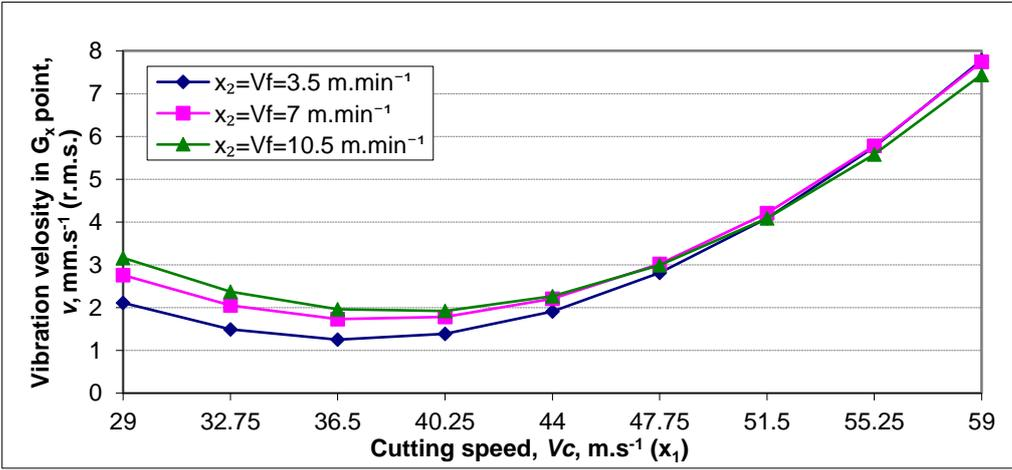
Fig. 5 Assessment of vibration velocity  $v$  at measurement point  $G_x$  in relation to the cutting speed  $V_c$  at different feed speed  $V_f$ .
