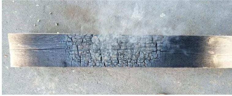
**Fig. 4 Sample treated with flame retardant HR prof after thermal loading.**
