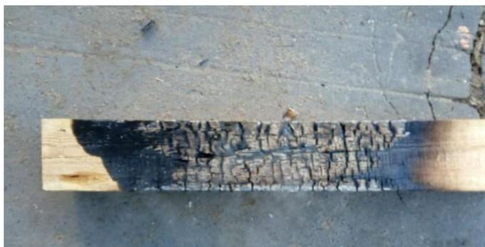
Fig. 6 Control sample, with no treatment, after thermal loading.
