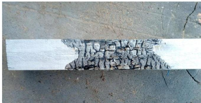
**Fig. 5 Sample treated with Striebrenka after thermal loading.**
