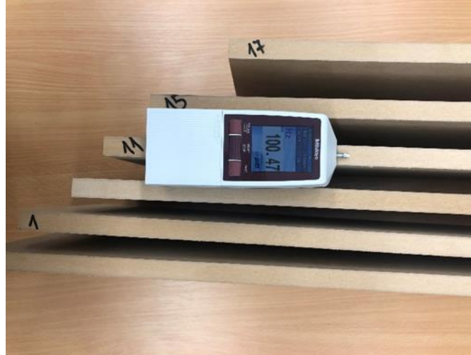
Fig. 3 General appearance of the a portable measuring instrument for surface roughness, model SurfTest SJ-210.
