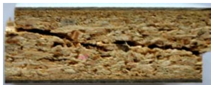
Fig. 5 Shear failure in the PBL central layer.
