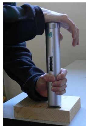
Fig. 2 System of penetration of working pin into wood in PILODYN
