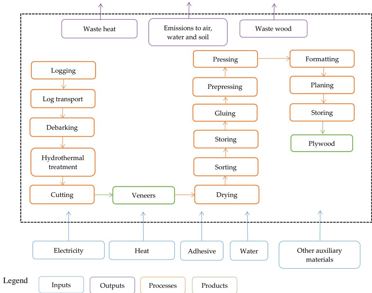
**Fig. 5 Simplified plywood production scheme.**
