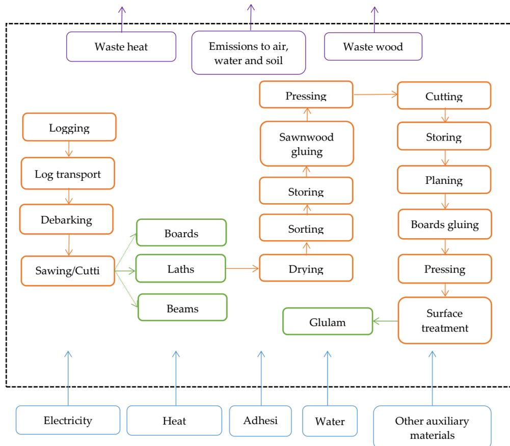
**Fig. 4 Simplified glulam production scheme.**
