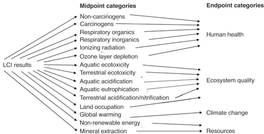
**Fig. 3 Overall scheme of the IMPACT 2002+ framework (JOLLIET *et al.* 2003).**
