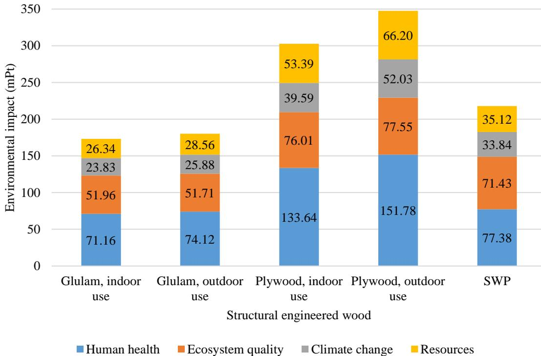
**Fig. 8 Single score of selected structural engineered wood.**
