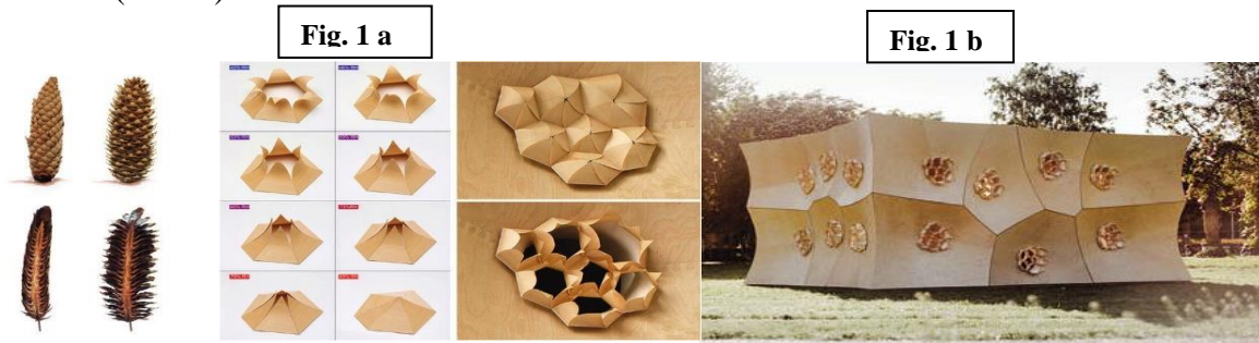
Fig. 1. a, b: The transfer of the biological principle of shape change triggered by hygroscopically induced dimensional change to humidity responsive, veneer-composite elements.
