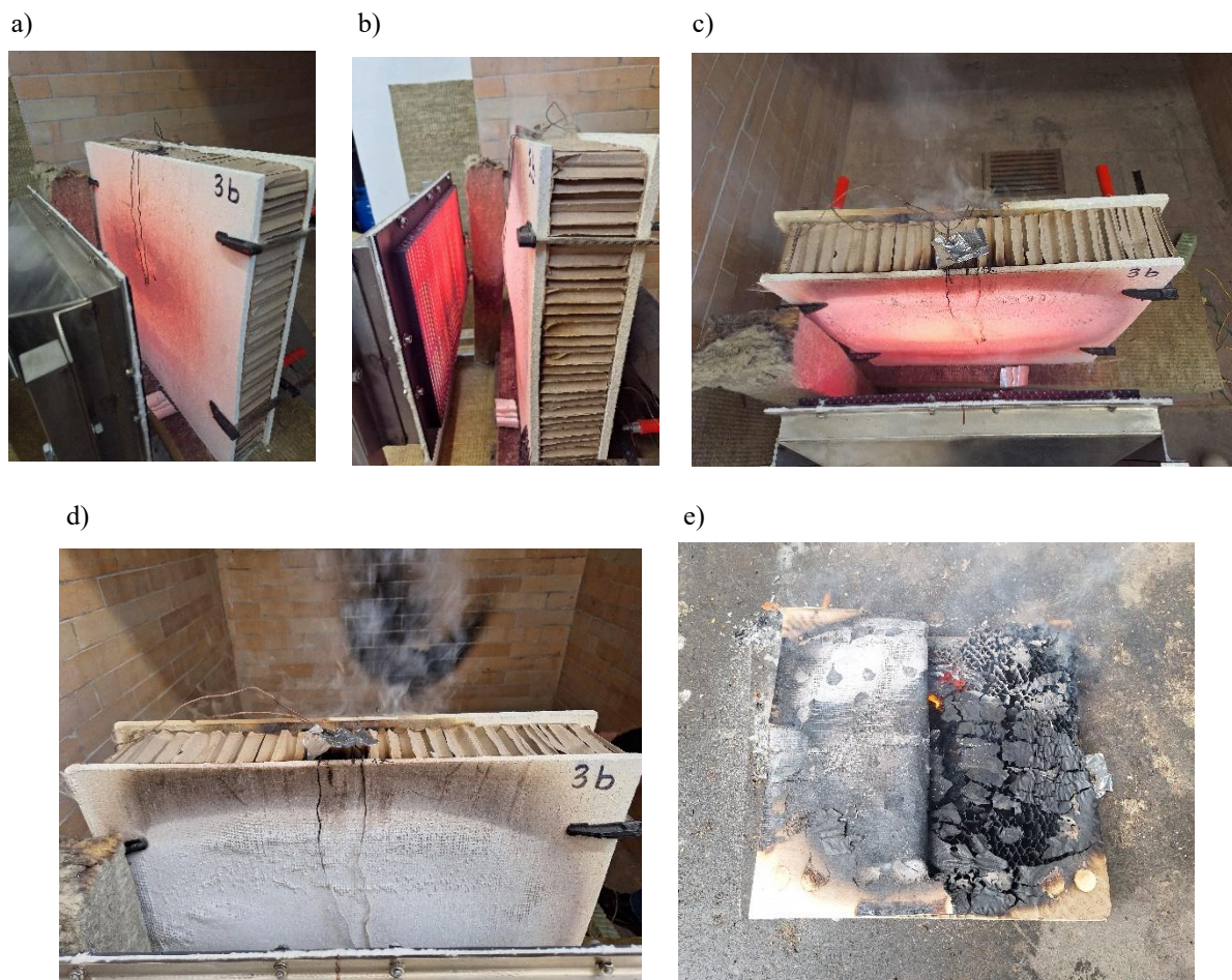
Fig. 13 Sample 2a (MgO–Honeycomb) during and after testing
